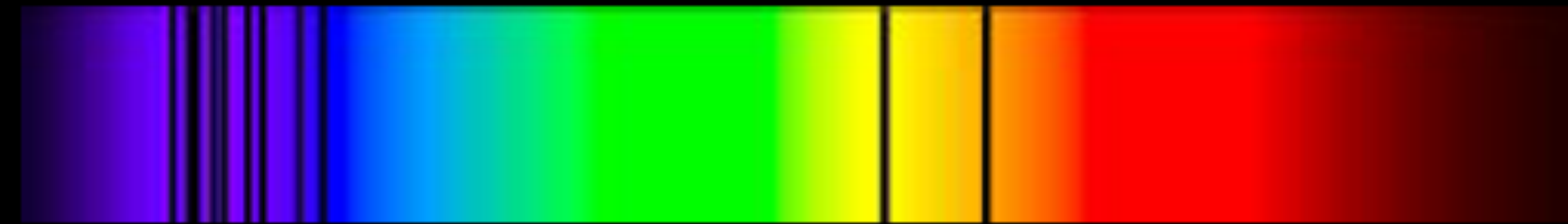
Absorption spectrum of sodium (Na)
