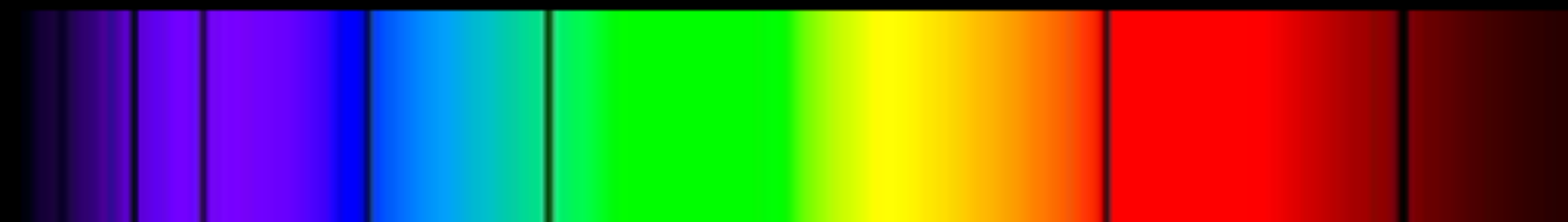
Absorption spectrum of lithium (Li)
