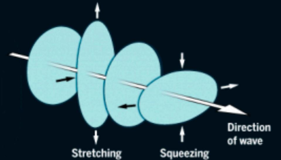
LIGO has detected waves of wavelength roughly equal to the distance between the detectors. The waves stretch each detector by about 1/10,000 the width of a proton.
